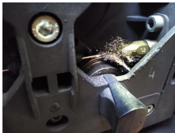
Picture-1 Excessive drive roll pressure may cause the copper coating to be scrapped off
