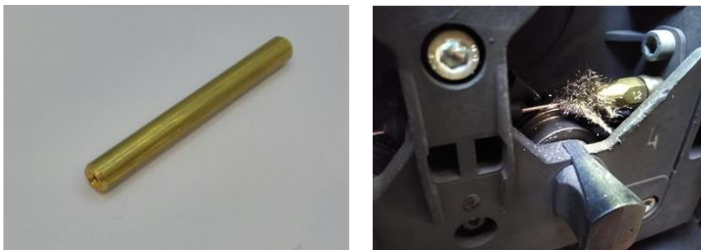
Picture-4 Left: wire guide Right: chip formation
