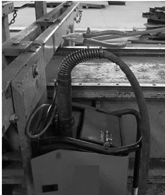
Picture-6 Excessively bent torch, wrong torch form
