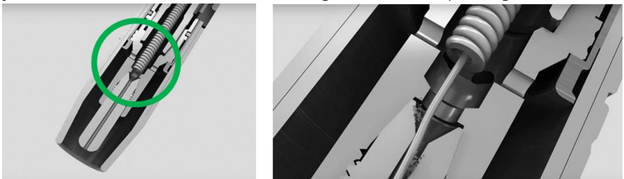
Picture-5 Left: mounting the liner correctly Right: too short liner is mounted
