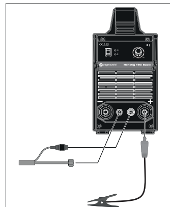
Figure 4 : TIG Welding Connections
