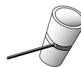
Pipe Fixed as Angle of 45° Inclined Position Welding Upwards H-L045 / 6G
