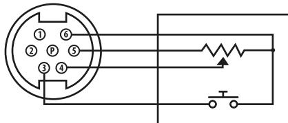
(3) Soldering direction has been taken as the reference.
