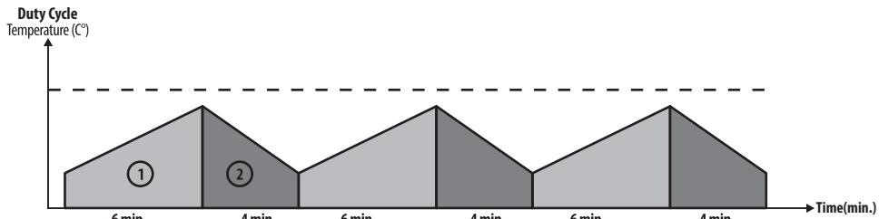
As defined in the standard EN 60974-1, the duty cycle rate includes a time period of 10 minutes. For example, if a machine specified as 250A at %60 is to be operated at 250A, the machine can weld without interruption in the first 6 minutes of the 10 minutes period (zone 1). However, the following 4 minutes should be kept idle for the machine cool down (zone 2).
